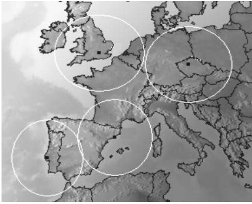
Figure 2. Example of Co-Channel Frequency Allocations with VDL Mode E
